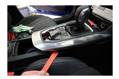
With the centre console lifted up, the two screws at the bottom of the radio are accessible. Remove these two screws.
