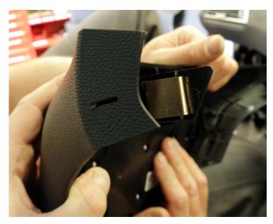
With the radio unit removed the air vents now need to be removed.
