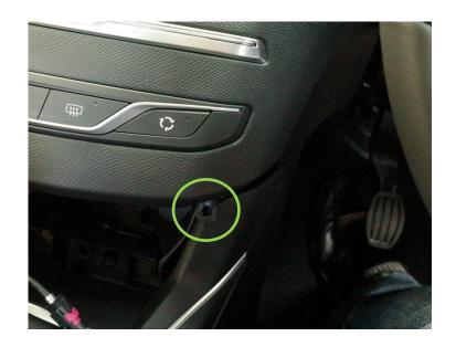
The top of the radio unit is held in by clips. There are two small slits at either end of the radio unit, use a radio removal key to push through the slit and release the clips. Note: the right hand side by the steering wheel is tricky to access, bend a stereo release key to a 90° angle to release this clip.
