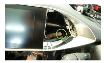
To the left air vent is harder to access, prise up the bottom of the air vent and shine a torch in and look for a felt strip.
