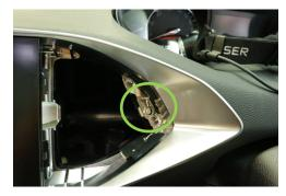
Finally, release the screen and silver trim that is held in by 4 spring clips, two at either end of the touch screen.
